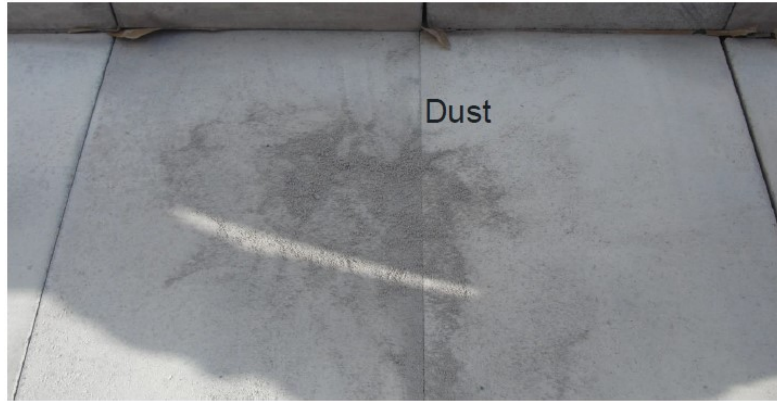
Figure 3. High level of free dust observed in tested low quality SiC slab.
