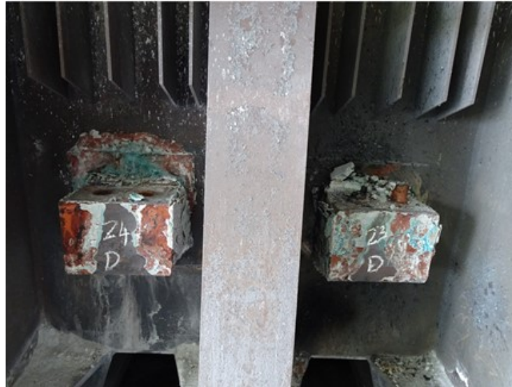
Figure 6. Collector bar attack by Sodium ooze.
