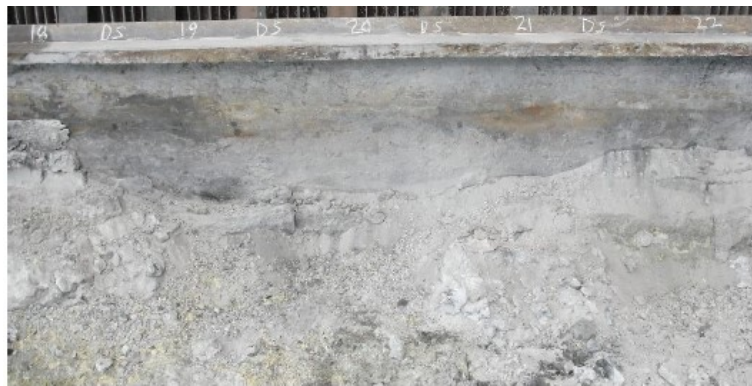
Figure 1. Highly reacted sidewall SiC bricks at lower cell life.
